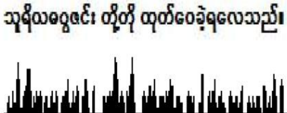
Fig. 6 Wrong Segmentation Error with Projection
